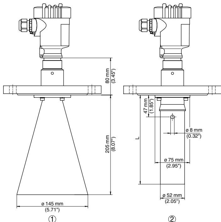
1 Version with horn antenna ø 145 mm
